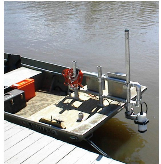
A boat-mounted ADP allowed Erick Swenson and his colleagues to conduct cross-channel transects at four depths, exploring differences in water movement at four depths and across channels. The team developed rating curves using the transect data and USGS synoptic data.
