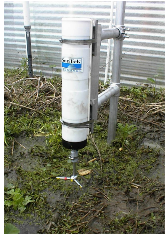
Slow-moving systems have long been a challenge to study. ADVs allow researchers to collect data on three-dimensional movement.
