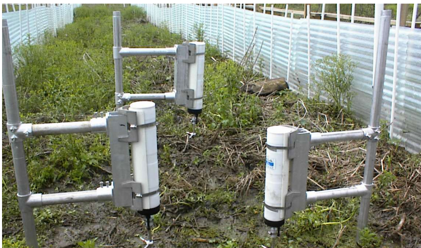
A flume built for a study on nutrient uptake shelters three ADVs that LSU scientists used to study the movement of water and sediment through Louisiana's Caernarvon Diversion. Pulse-coherent technology offers highly accurate readings even in extremely shallow or slow-moving water.
